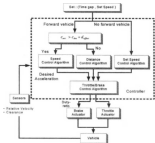
Fig. 2 Vehicle longitudinal control algorithm
